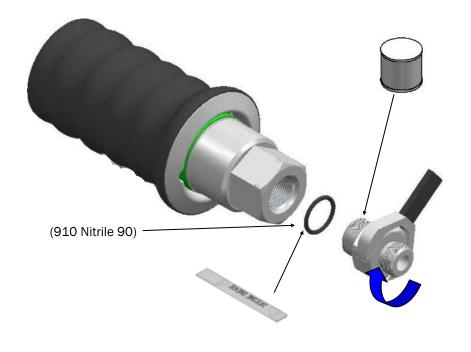
Torque the nozzle to 90Nm when tightening
