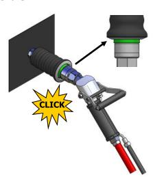
3. Open the handle on the fill valve to begin filling
