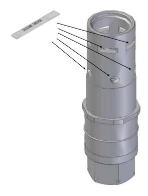
8. Insert NC104 tool into the nozzle, and insert sleeve spring.
